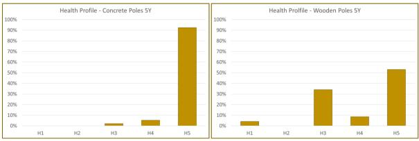
Note: This includes the 110kV concrete and wood structures, but excludes the 110kV steel towers & privately owned poles.
